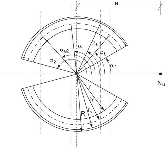
Figure 1. The cross-section weakened by two openings
