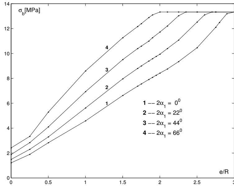
Figure 3. Stresses in concrete  $\sigma_b$  versus eccentricity ratio  $e/R$  and size of opening  $2\alpha_1$
