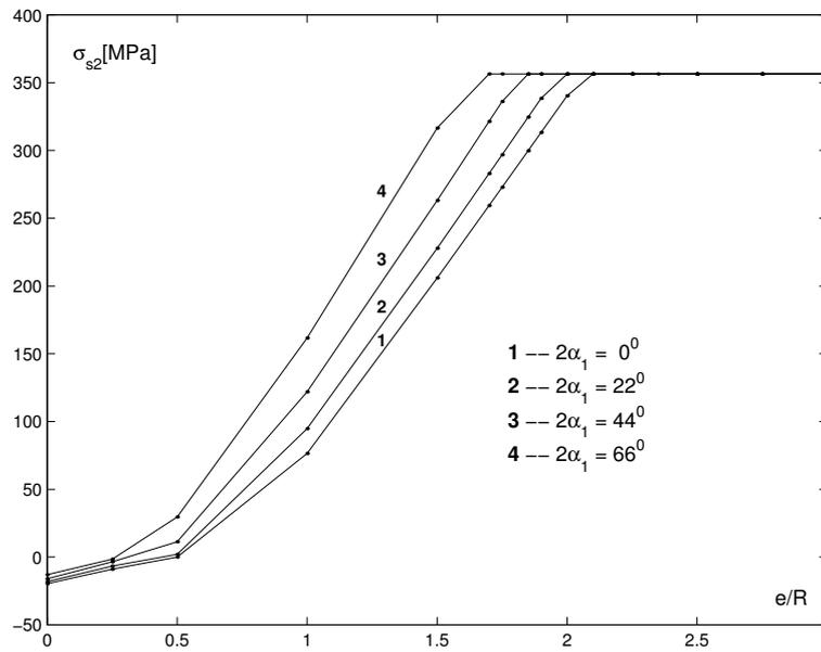
Figure 4. Tensile stresses in steel versus eccentricity ratio  $e/R$  and size of opening  $2\alpha_1$
