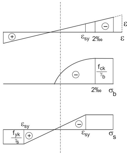
Figure 2. Distribution of strains  $\epsilon$ , stresses in concrete  $\sigma_b$  and in steel  $\sigma_s$  across the section
